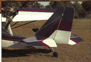
Steering is provided by the Maule tailwheel, which releases to full caster.
