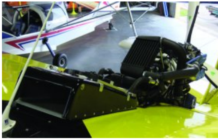
In the Searey installation, the 915 iS requires a radiator with a scoop. The intercooler is immediately behind it angled into the slipstream.
