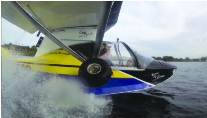
The higher power of the 915 iS, above, gets the Searey off the water in about 11 seconds, two seconds faster than the 914-powered version.
