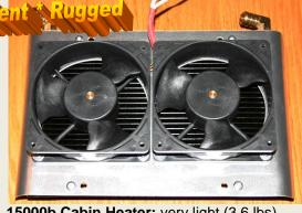
15000b Cabin Heater: very light (3.6 lbs) 15,000 BTU. Hi flow fans (130 and 260 cfm) High efficiency aluminum shroud. With 90 degree fittings for 5/8 heater hose. Stocked item
