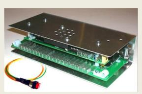
ACI SeaRey Power Buss: 12v DC overload monitoring and protection for 18 circuits +2. Warning light and voice annunciator identifies overloaded circuit. Avionics starter protection. Raises the standard! Searey
