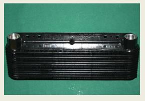
Oil Cooler: for Rotax 912, 912s and 914. Aluminum. (NPT fittings not supplied.) Size: 11" x 4.75" x 1.5" 12 plate, 7500 BTU Stocked item US\$39
